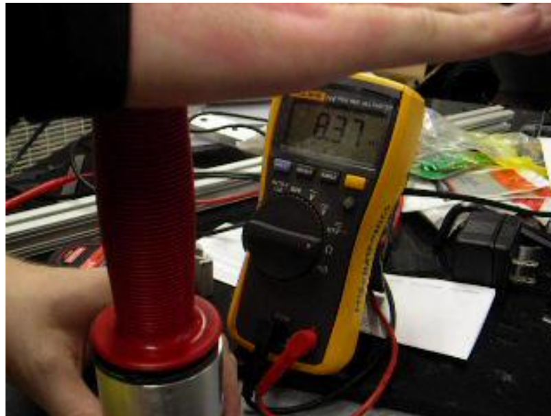
Mounted potentiometer displacement response (video)
